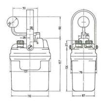
All electrical parts and the complete blasting machine are tested with a tension of 2000 V A.C.
