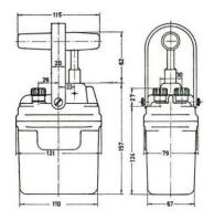
All electrical parts and the complete blasting machine are tested with a tension of 1500 V A.C.
