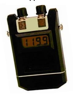
Measuring range: 0,0 – 2000 (1999) Ohm Measuring current: max. 0,3 mA
